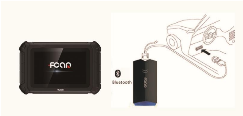
Figure 3.2-2 Connection of non-OBD-II interface
